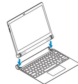
**Align the keyboard slots with the tablet connectors and insert the tablet into the keyboard.**
