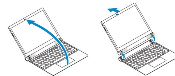
**Turn the tablet outward to disconnect the keyboard.**
